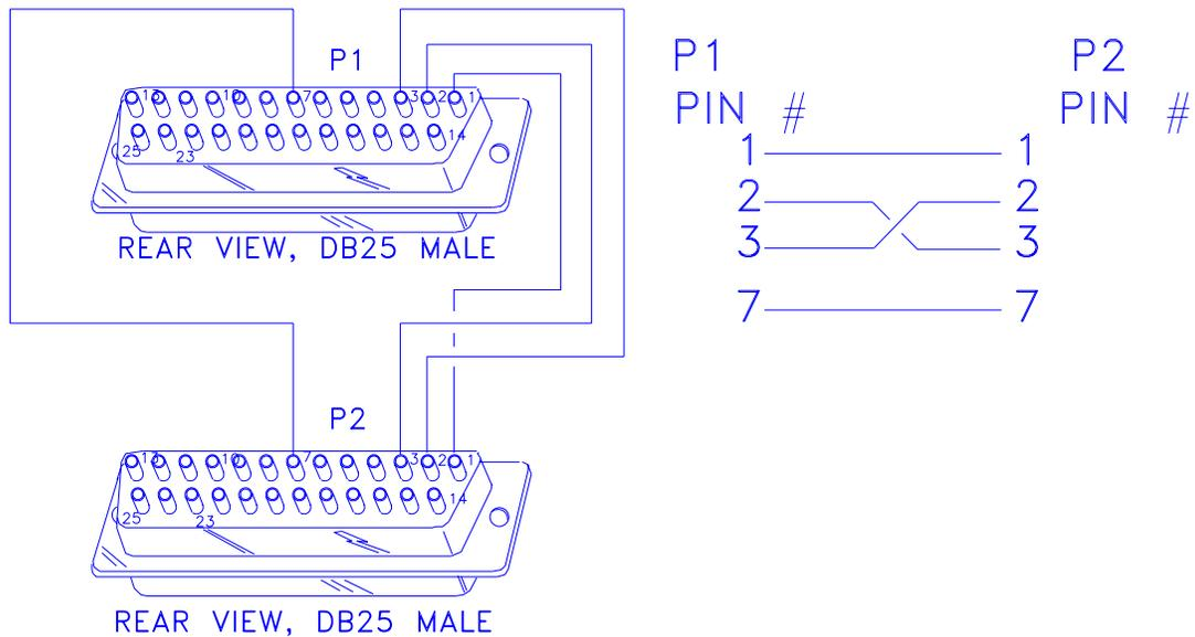
The configuration shown here will enable two KPC/KNET nodes to gateway between two or more frequencies or baud rates. If more baud rates or frequencies are needed for gateway connectivity, the diode matrix shown below may be utilized (Drawings by BuckK4ABT). For more info, visit: [www.SEDAN.org](http://www.SEDAN.org)
