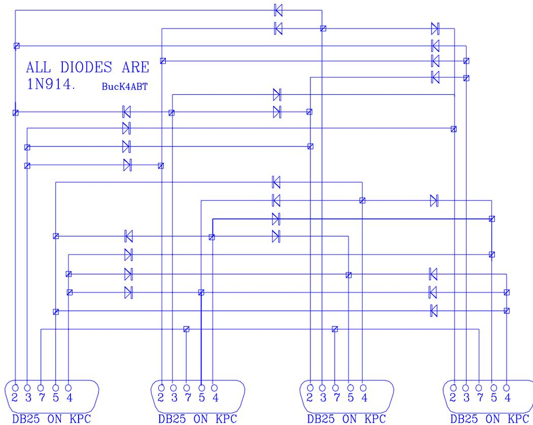
A diode matrix is used to “stack” more than two KPC KNET nodes. A five port Diode Matrix follows the same logic as above, with six ports probably being about the limit of practicality. The number of diodes required for a Diode Matrix with  $N$  serial ports is  $2*N*(N-1)$  (Drawings by BuckK4ABT).
