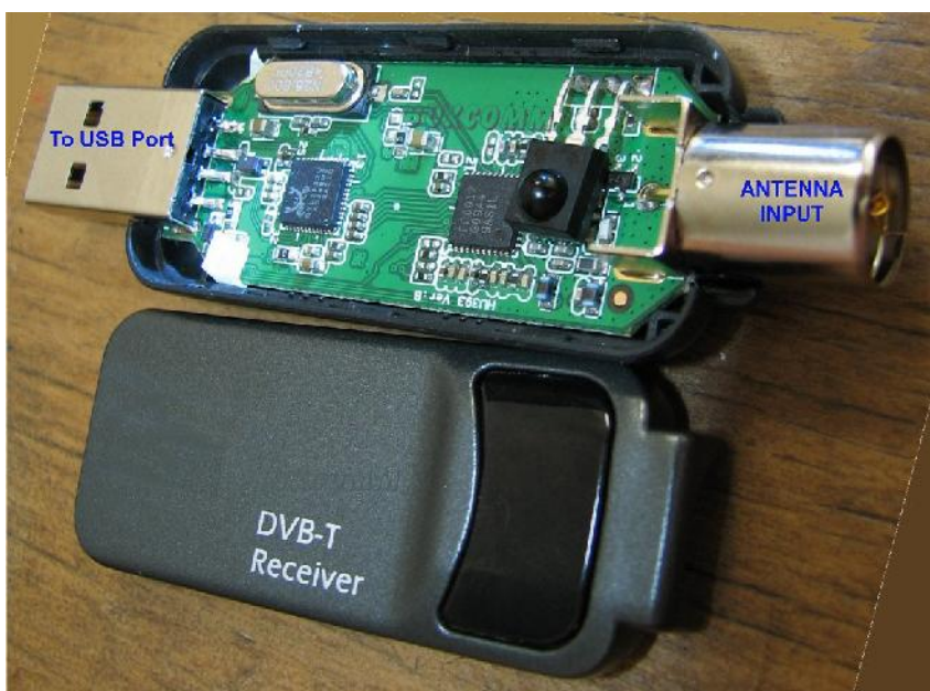
The photo above reveals the "wheels and whistles" within an SDR dongle, and the antenna input and USB output ports.
